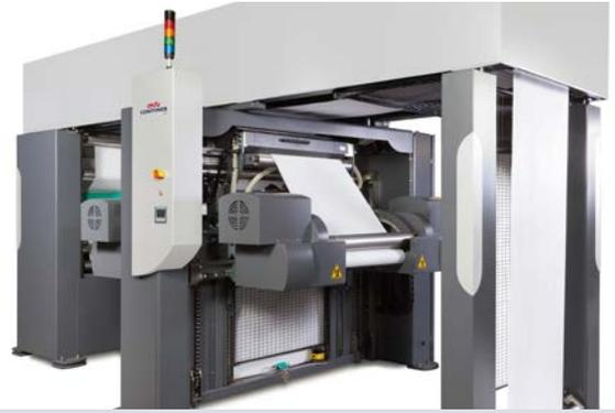
The reel change and web transfer to the new core is then automatic. As for all models, operational data is shown on the HMI of the rewriter and motorized reel sidelay is included as standard. Additional options are as for the CR-W.
